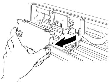
Use the procedure under "Installing the ribbon cartridge" on page 5 to install a new cartridge.
