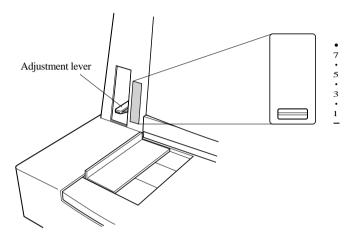
□ Move the adjustment lever to one of its nine settings. Position 1 is most suitable for single-sheet paper.
