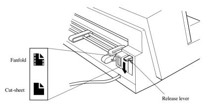
□ Set the release lever on the back of the printer to the fanfold position.
