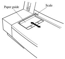
□ Making sure that the left edge of the paper is against the paper guide, insert a sheet of paper into the front of the printer.
